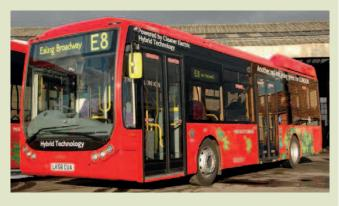
it: "Series hybrids are electric buses with diesel generators. As battery technology improves, we can downsize the diesel generator, or maybe use in-road induction charging or overhead lines, to supplement the charge."
