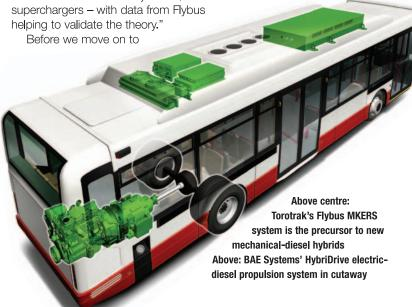
the future, note that Flybus used Allison's standard gearbox PTO. Hence the potential for adding mechanical KERS to existing buses. "Using the existing hardware infrastructure means that this mechanical hybrid technology is ripe for retrofit, using a relatively simple bolt-on assembly," explains Fuller. "That's a huge market."
